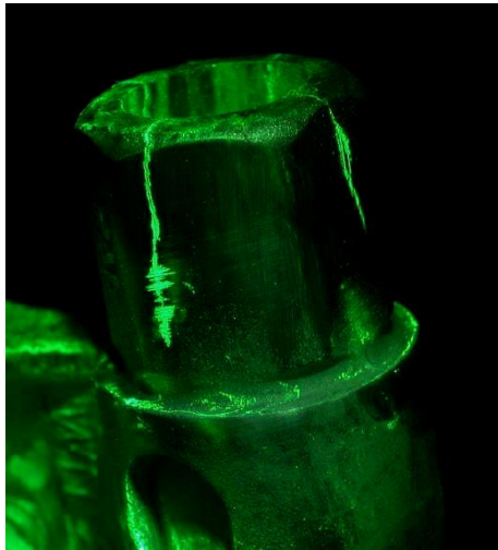
Fluorescent penetrant testing
