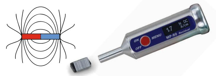
With the handy, battery-operated List-Magnetik MP-80 residual magnetic field meter, you can quickly and reliably determine the residual magnetism, also known as remanence, on ferromagnetic iron and steel parts. The measuring device can also be used to check demagnetized parts.
