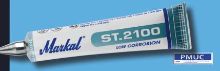
Markal® ST.2100 is a metal-ball tip marker that meets European nuclear requirements. The low sulfur and low chloride content allows for safe marking on stainless steel. The aluminum squeeze tube and thick paint makes it suitable for vertical and overhead surfaces.
