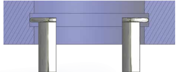
Messen einer Innennut Measuring of internal recesses
