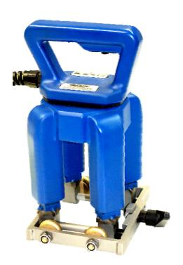
Two AC yokes (pole spacing 140 mm) are arranged crosswise. They are supplied by two equal AC currents at 90 degree phase shift. Thus, a rotating magnetization vector is created, whose field strength is equal in all directions.
