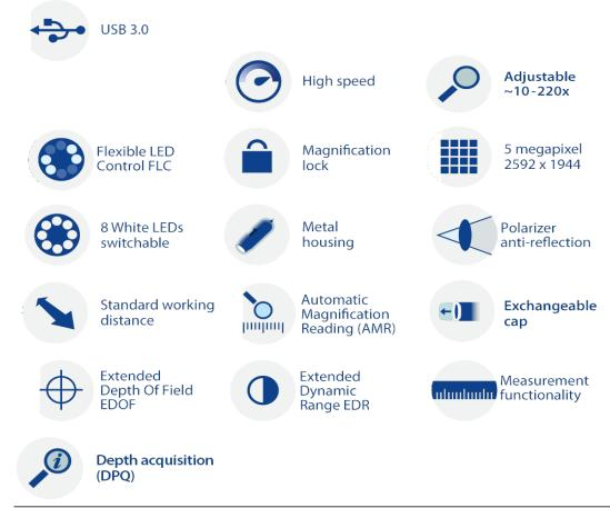
EDOF allows users to automatically capture multiple images at different depths and automatically combine them into one clear image. EDR automatically captures and combines multiple images at different exposure levels to produce a final image with greater dynamic range. The AMR function automatically detects and displays the magnification of the Dino-Lite. The magnification is displayed within the Dino-Lite software and stored with the captured picture and simplifies the measuring process.
