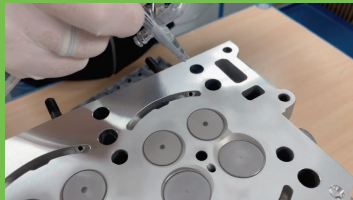
ATTBLIME AB6 G sprayed using air brush
