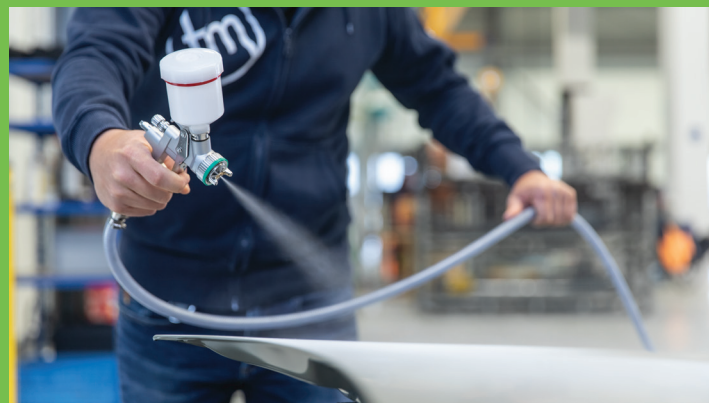
ATTBLIME AB6 G sprayed using spray gun
