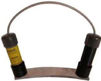
"Flaw-Finder": The easy way for the effective magnetization of components for crack dimensions and flaws.
