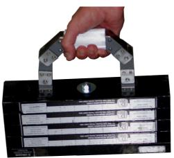
The permanent magnet Flaw Finder was created and tested according to ASTM E709-95 & ASTM E1444. The magnetizing force of the permanent magnet was tested by determining its lifting power on the TB-10 magnetic weight lift test bars. The lifting force relates to the magnetic strength of the permanent magnet. Herewith we certify that the permanent magnet Flaw Finder has lifting
