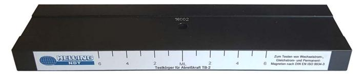
Test body TB-2 for testing and calibration of lifting force of hand yoke magnets.
