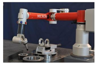
**MICRON** is light-weight and have an easy handling, the counter-balance makes the movement of the axes extremely smooth. The operator holds the probe and guide the arm supporting only 15grams weight.
