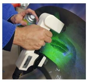
The light sources can be fixed quickly and easily to the yoke leg and fastened with two plastic screws.
