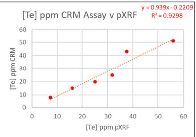
Fig. 4. Tellurium (Te) performance demonstrated on OREAS 600 series CRMs . 50kV performance for Te is generally inadequate to allow definition of anomalies due to it being often present at low concentrations.
