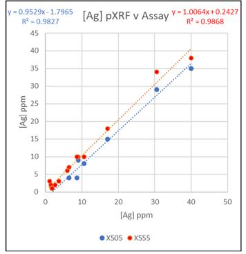
Fig. 3. Ag performance improvements are obvious both in relation to lower detection limits and improved accuracy. In addition to being a valuable primary target element, it is also important in Au and base metal systems as well.
