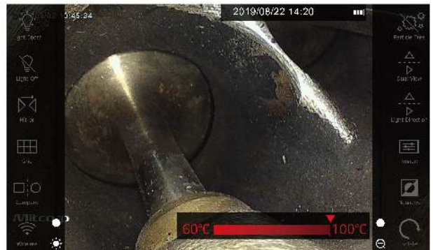
3 stage temperature warning & auto shut-down function
